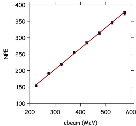
Figure 1: The number of photoelectrons per end of the BCAL module as a function of energy.
