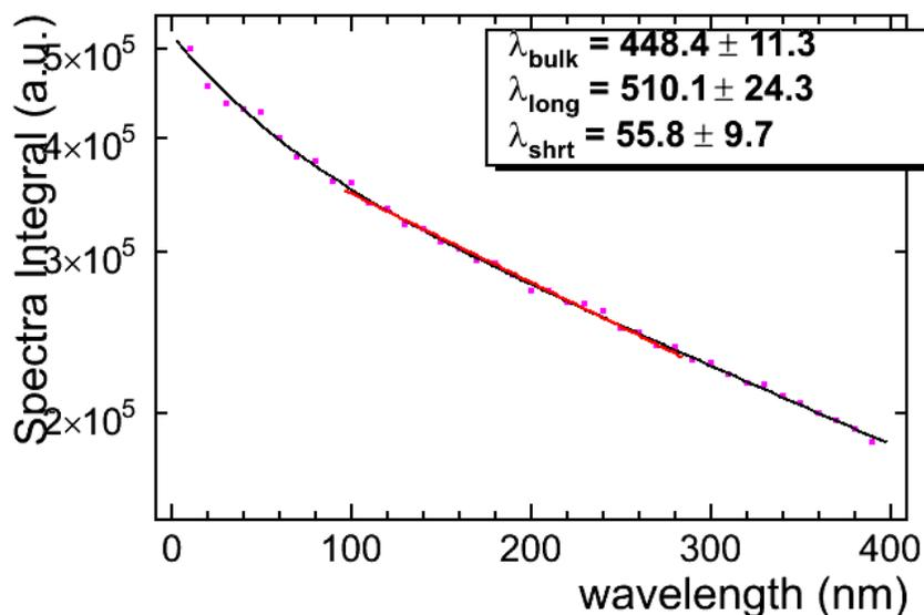
Fig. 3. Integrals of the Moyal fits to the fitted data are plotted as a function of source distance for Fibre 09-3. The curve is a results of a fit to a double exponential (shown in black). The bulk attenuation was extracted over the distance range of interest (shown in red), as specified by Kuraray. The legend shows it as well as the short and long attenuation components found using a double exponential fit.
