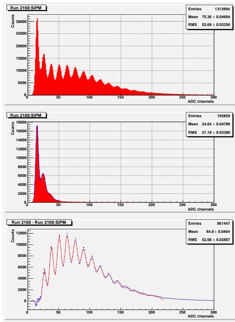
Fig. 4. Raw ADC spectrum (top), pedestal spectrum (middle) and subtracted spectrum and fits (bottom). Details are provided in the text.
