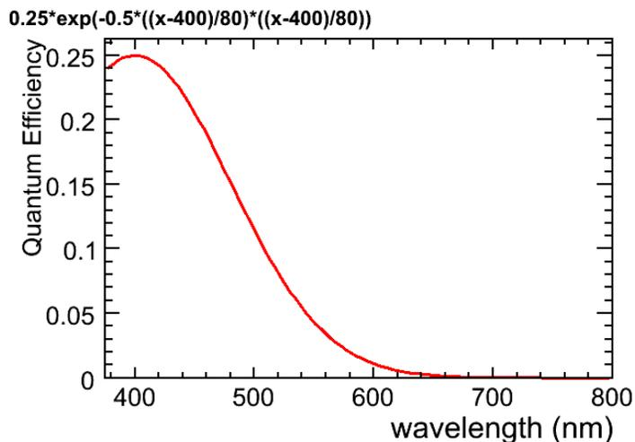
Fig. 1. Quantum efficiency parametrization versus wavelength, using Eq. 2. This curve was folded with the raw data to produce spectra more directly comparable to those of Kuraray.
