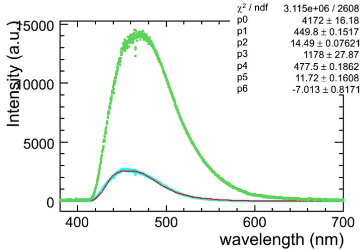
Fig. 2. The green data points are the raw spectra as seen by the photo-spectrometer. The light blue points are scaled by an approximation to the quantum efficiency of a bi-alkali photocathode. The fit functions were of the double Moyal type.
