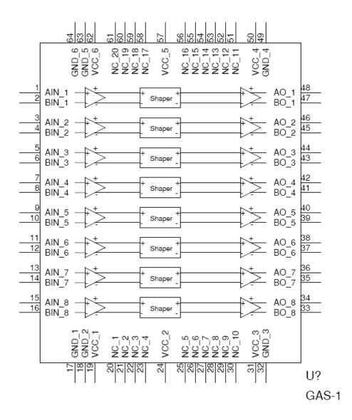
Note: NC pins (No Connect) are not yet assigned.
