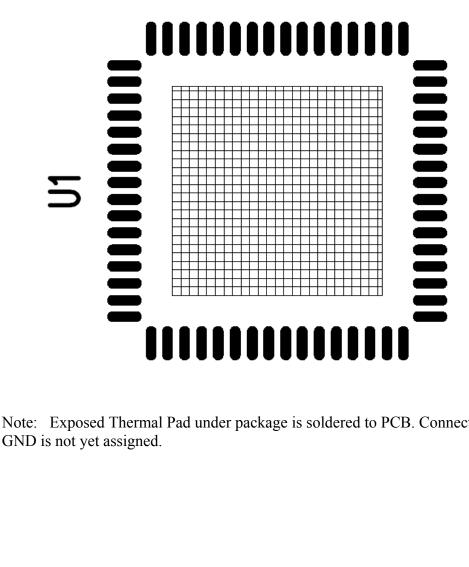
Note: Exposed Thermal Pad under package is soldered to PCB. Connection to VCC or GND is not yet assigned.
