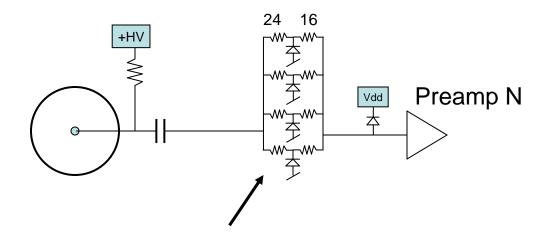
Intended to withstand .1 - .5mJ discharge spikes. We expect that the board desigh will retain space for external protection unless fabbed devices are shown to meet input protection requirements.
