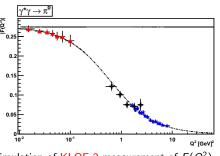
Simulation of KLOE-2 measurement of  $F(Q^2)$  (red triangles). MC program EKHARA 2.0 (Czyż, Ivashyn '11) and detailed detector simulation. Solid line: F(0) given by chiral anomaly (WZW). Dashed line: form factor according to on-shell LMD+V model (Knecht, Nyffeler, EPJC '01). CELLO (black crosses) and CLEO (blue stars) data at higher  $Q^2$ .
