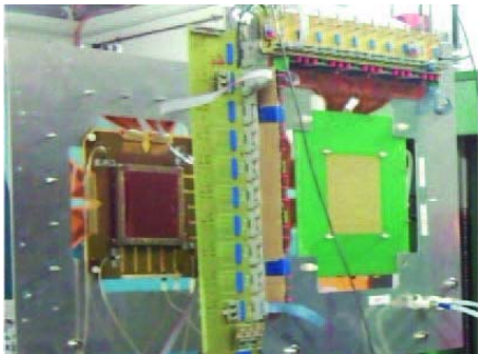
Figure 2: GEM chambers of the prototype tracker being prepared for the beam tests during hall A PREX experiment.
